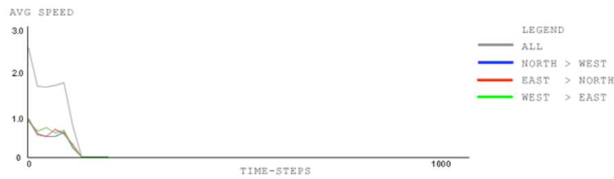
Figure 18. signal-type: All-Green; wait-time-limit: 120 time-steps; car-density: 1.0, plot-window: 20 time-steps
